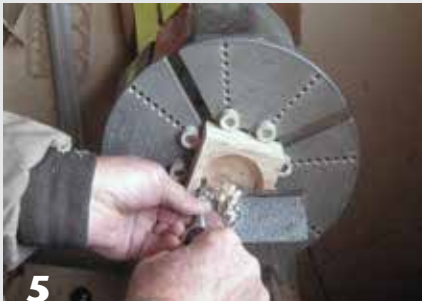
5 The box cavity can have straight or sloped sides, depending on your preference.
