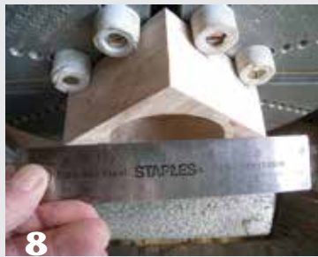
8 The author uses a sharp hand plane blade as a scraper, then checks for flatness with a straightedge.
