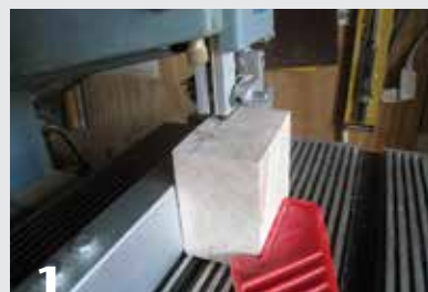
1 Cutting the lid from the box blank ensures continuous grain flow from lid to body, as well as uniform sizing of parts.
