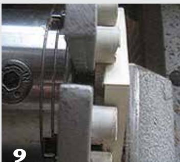
9 When mounting the thin lid part, position a spacer behind it so its surface protrudes above the holding buttons on the chuck.
