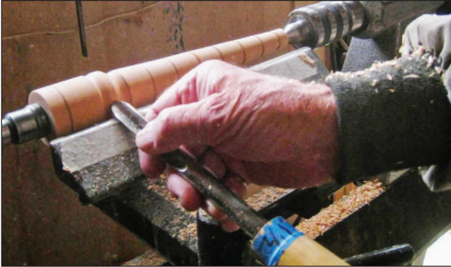
5. Use a spindle gouge to create the simple bead between the shaft and handle.
