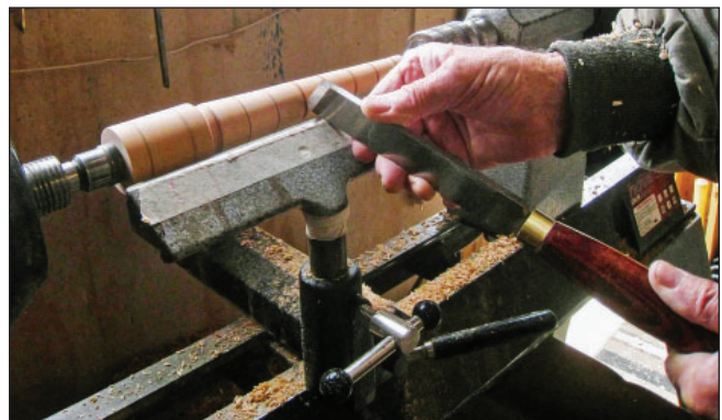
4. Use the long point of the skew to define the planting depth marks on the shaft.
