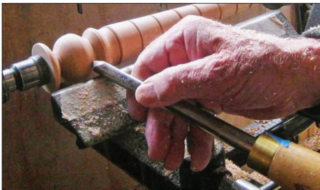
7. Round the corners created by the coves to create the large bead form comprising the handle.
