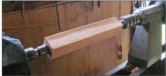
1. Securely mount the blank between centers using center-punched holes for alignment.
