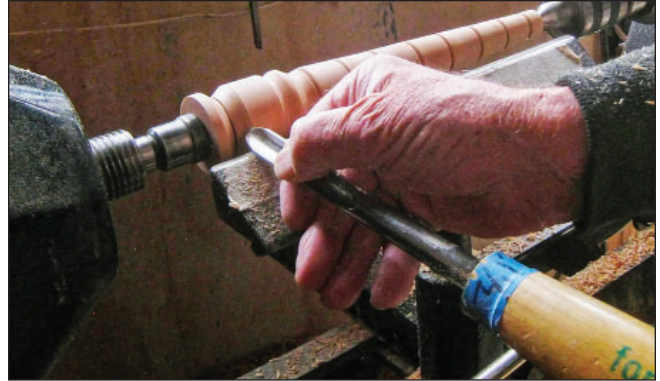
6. Cutting a cove on either side of the handle quickly removes waste and creates space for subsequent tool movement.
