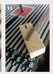
The veneer should slide into the kerf with little or no force.
