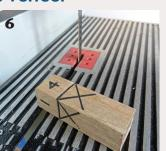
Glue your veneer in place and allow the adhesive to cure. After curing, trim the veneer flush with the surface of the blank. After cutting and inlaying veneer in all four sides, your blank will resemble this example. Here the lines are drawn but not yet cut.
