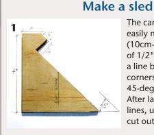
The carrier sled is easily made from a 4"-(10cm-) square piece of 1/2" plywood. Draw a line between two corners to find your 45-degree cut line. After laying out your lines, use a bandsaw to cut out the jig.
