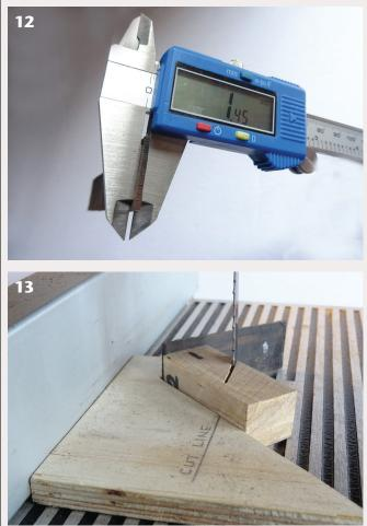
If you find your veneer is prone to crumbling, try cutting it a little thicker. Use a piece of the veneer to offset your blank for a second cut to widen the kerf.
