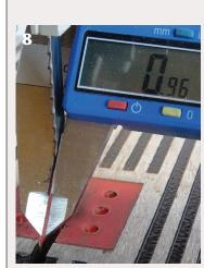
Measure the thickness of your bandsaw blade—this should be the same as the resulting kerf.
