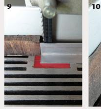
A thin cut between the blade and the fence can be dangerous, and you risk the blade hitting the fence—better to have the veneer peel off the outside of the cut. Hunt around your shop for a proxy that will help you quickly setup thin veneer cuts, such as a piece of aluminum angle stock.
