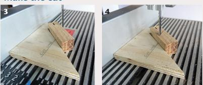
Place your blank against the hook in the carrier sled and cut a kerf for the veneer, stopping about 1/8" of short of a through-cut.
