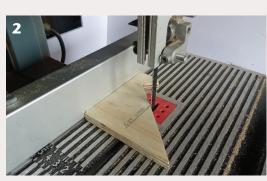
Use your carrier sled to setup your cut. Set the fence so that the bandsaw blade aligns with the designated cut line on the blank.
